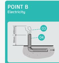
Connected to the power network 03. 3 cables 2,5mm<sup>2</sup> 04. Corrugated flexible conduit Ø20mm
